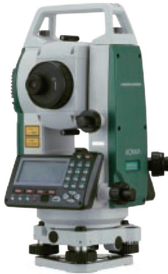
Gambar 3 Contoh Alat Total Stasion
